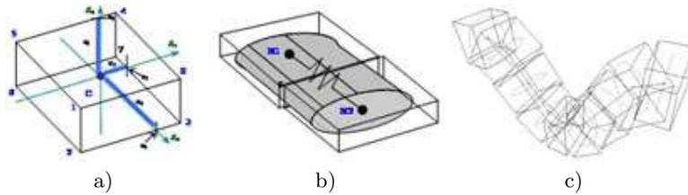
**Figure 3.** Bounding volumes in the model: a) an OBB; b) CP bounded by OBBs; c) yarn bounded by OBBs.
