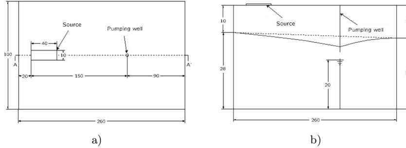
**Figure 1.** Plant and section views of the flow domain (dimensions are expressed in meters).
