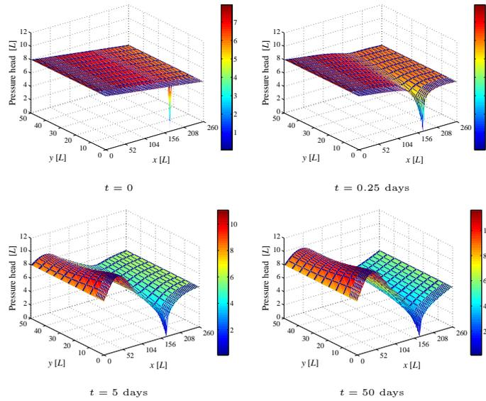
**Figure 2.** Evolution of the pressure head  $\psi$  at the plane  $z = 20$ .
